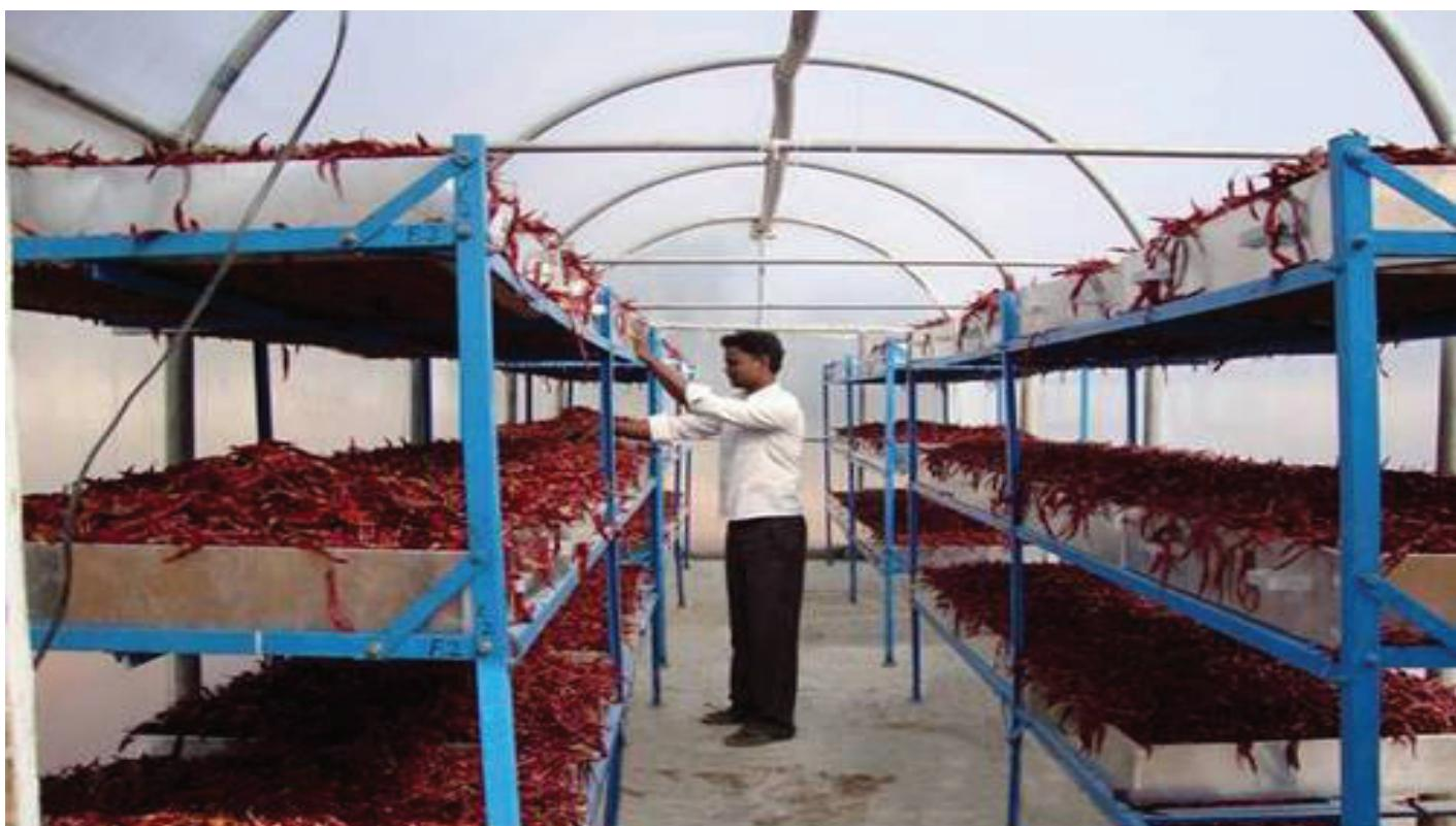
**Chilli drying in Solar Tunnel Dryer**
